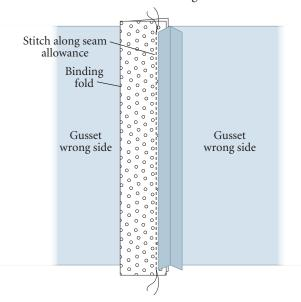
Press flat, and then press the binding over, covering the open flat seam allowances.
